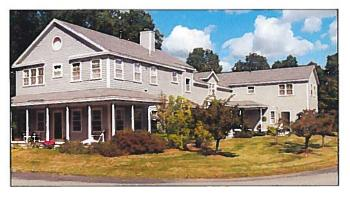
below, multi-pane above, banded and grouped windows, and recessed windows. Strips of three or more windows, commonly called banded windows, may be an effective way to enliven the rigidity and repetition of regularly spaced single windows and to bring large amounts of light and ventilation to the interiors.
